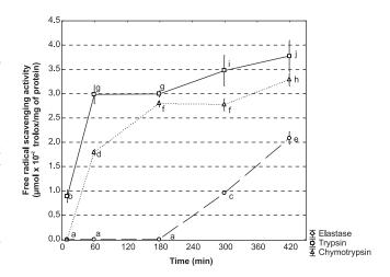
FIGURE 4. Free radical (DPPH) scavenging activity of enzymatic hydrolysates of EWPP (egg-white protein precipitate). The hydrolysates prepared with (O) elastase, ( $\Box$ ) trypsin, and ( $\triangle$ ) chymotrypsin (a,b,c...-the same letter in indices of means shows no significant differences at p≤0.05).
